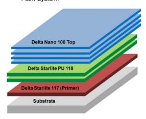
As self-cleaning coating for painted surfaces of building façade and mineral surfaces such as ceramic tiles, roof tiles, marble, granite, stone, concrete, masonry.
